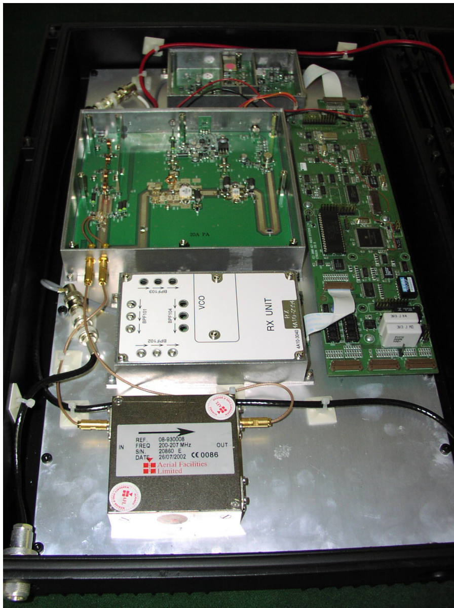
Fig.1 Storno CQF9000, Case Remilled, New Key Modules in Place, Screening Removed
