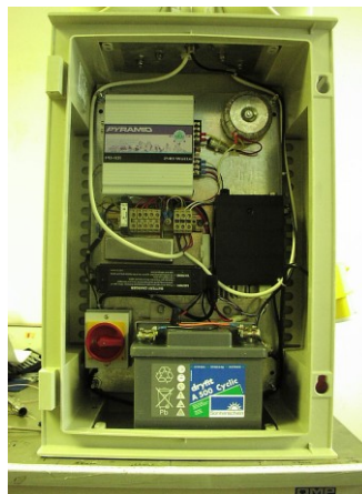
Fig.6 Wireless PA Outstation, Cover Removed for Bench Testing
