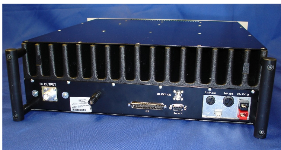
Fig.4 Key 100Watt POCSAG Paging Transmitter, Rear View Showing Heatsink Casting
